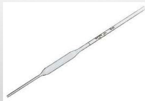
Glass pipette used to accurately measure specific, set amounts come in various sizes.
